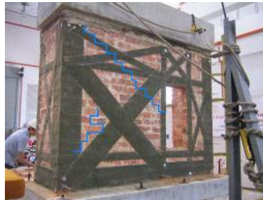
(a) PGA = 0.35 g: Cracks patterns
