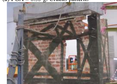
(c) PGA = 0.80 g: Upper portion collapsing
