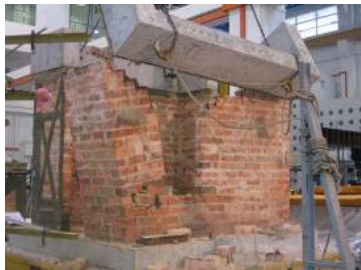
(c) PGA = 0.35 g – The left portion toppling
