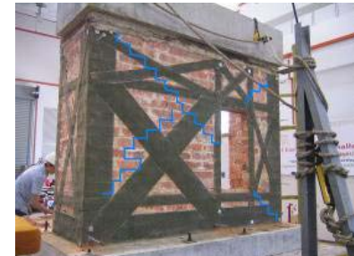
(b) PGA = 0.45 g: Ultimate crack pattern
